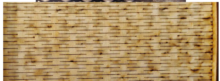
Kerf cutting pattern (short, offset lines)
